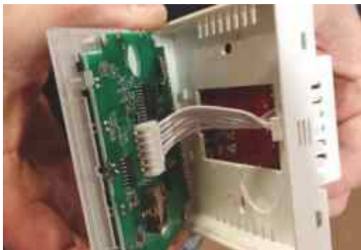
3. Front and rear circuit boards are connected with the control wire.
