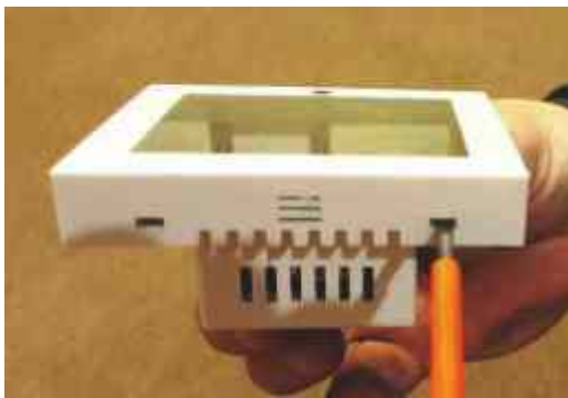
1. Insert small flat screwdriver into slots to unclip screen release lugs.
