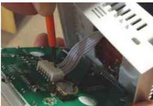
4. Carefully unplug control wire from front circuit board
