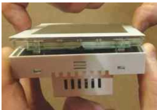
2. Carefully remove screen and front circuit board.
