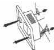
Fix back using screws provided.
