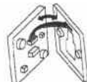
Re attach control wire to screen.
